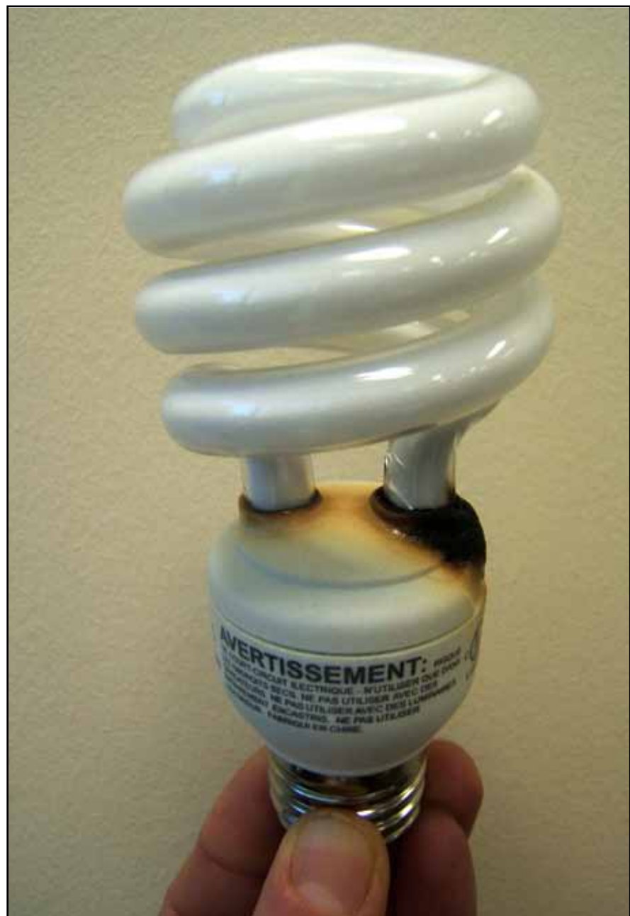
BURNED OUT... The burned area at the base of this compact fluorescent lightbulb shows that it has ended its life properly, and is a normal part of the process.
